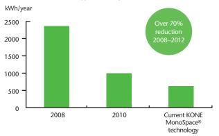
The basis for the calculation is an elevator speed of 1 m/s, a load of 630 kg, 150,000 starts/year, a travel height of 9 m and 4 floors
