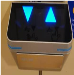
Car Operating Panel or Hall Call Button Able to replace all types of buttons
